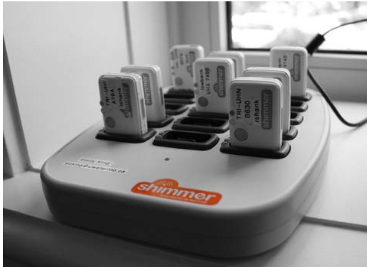
Inertial Measurement Units, which track personal support worker body motion.
